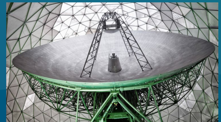
Space observation radar TIRA/Fraunhofer Institute for High Frequency Physics and Radar Techniques FHR/Fraunhofer FHR © Fraunhofer FHR
